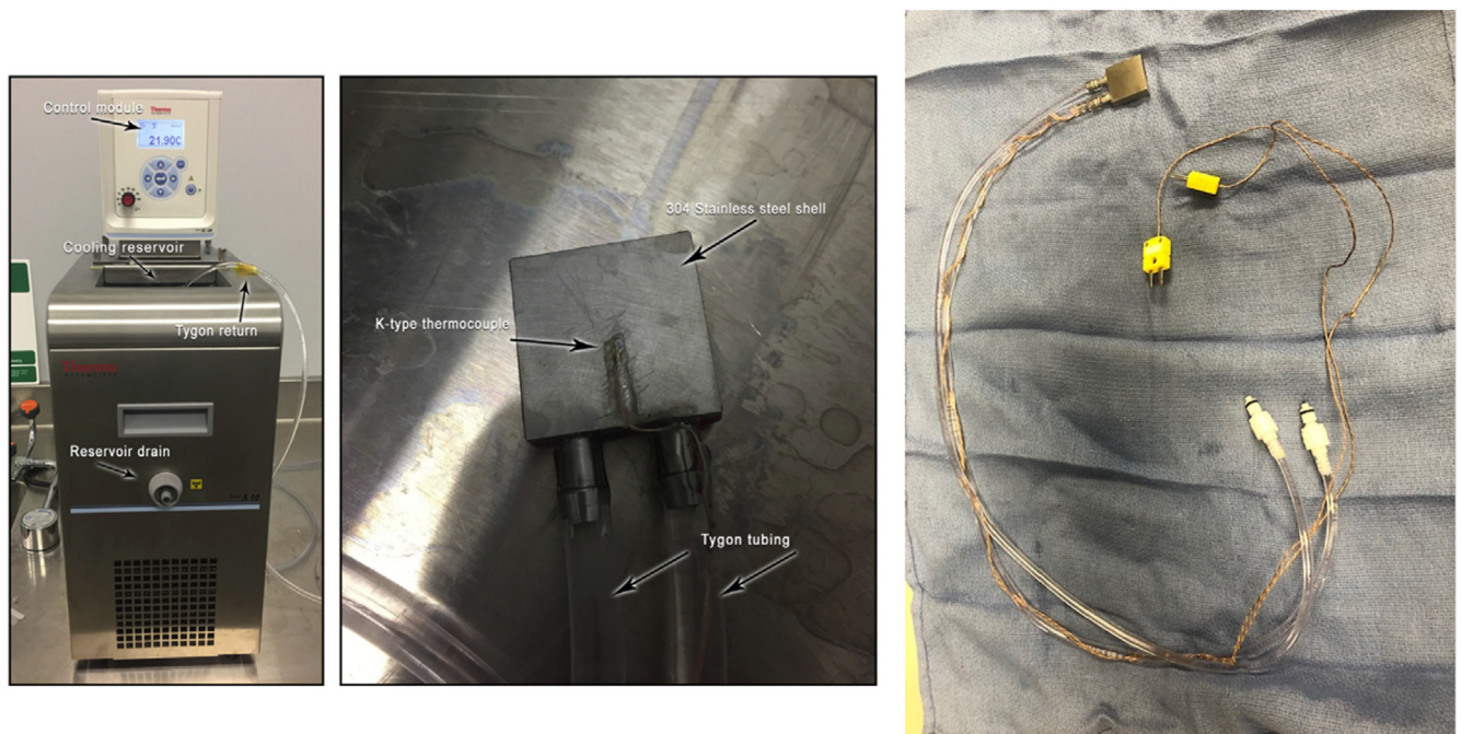
Figure 2 Equipment used to cool the oblique sinus during cardiac surgery. (Left) Chiller kept at bedside that cooled saline and pumped it through the system to maintain a specified temperature at the posterior left atrium. (Middle) Close-up of the cooling element through which saline circulated. (Right) View of the cooling elements with tubing, snap connectors for fluid, and electrical connectors for continuous temperature monitoring. Modified with permission from Witt et al. 11
